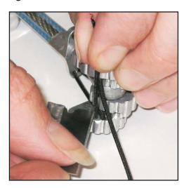
14. Trim the extra cord flush to the surface of the cam lobe. Be very careful to cut only the extra cord without cutting into the trigger cord. If you accidentally cut the trigger cord, you must remove it and start over. Be very careful not to pull on the trigger after you have cut the extra cord, because it will pull out of the cam lobe.
