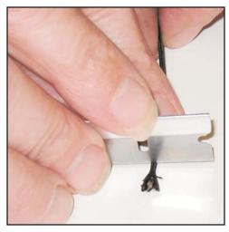
4. Cut two 15cm pieces (6 inches) of cord. The Kevlar core will not melt when heated, and is very hard to cut. Use a sharp razor blade to make very clean, precise cuts.
