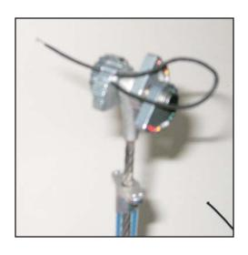
9. Route the cord back through the top hole then pull gently so that it nests down into the slot, but does not pull through the first hole.
