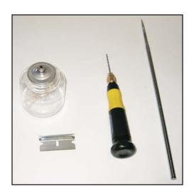
The replacement process is quite simple, and requires only a #50 drill bit, a candle, a small pick, and a very sharp razor blade.
