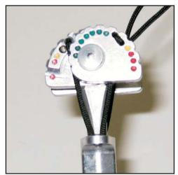
13. Adjust the length so the cam lobes are even, with no slack, but not too tight. If the cord is too tight it will pull the trigger assembly unevenly when the trigger is activated.
