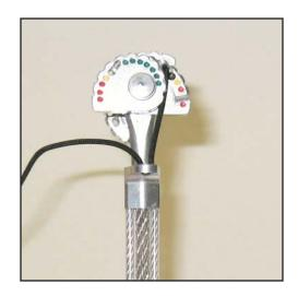
11. Adjust the cord so that when the cams are in the open position and the trigger piece is tight to the end fitting, the cord is straight and tight.
