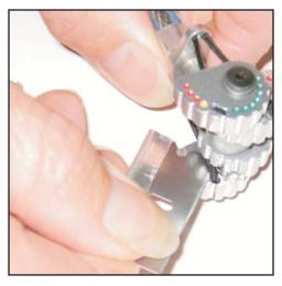
1. Cut off the old cords as close to the cam as possible using a sharp razor blade.
