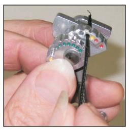
7. Starting on the inside cam, route the cord through the lower hole, pointed end first. This is the hole closest to the outside tip of the cam lobe.
