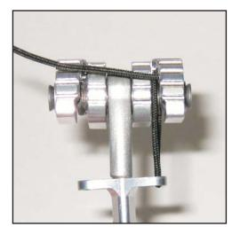
12. Pass the cord up to the outside cam lobe, and do the reverse cord routing as on the inside cam.
