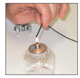
5. Heat the end of the cord until the black nylon sheath material begins to melt, then pull it quickly through your fingers to get a nice point on the end, with no core material showing. Repeat this several times to get a good point.
