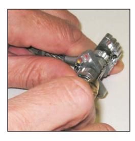
2. Remove the cord from inside the holes using a small drill bit (size #50, or 1.8mm).
