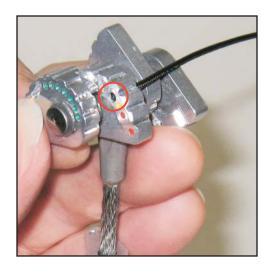
8. Pull the cord so that the melted ball end is lightly wedged into the hole, and is even with the surface of the cam lobe.
